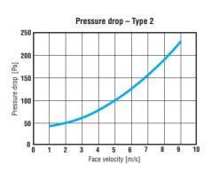
Typical pressure drop of a two-stage system type 2. Figures are valid for face velocity at operating point and for clean filters.
