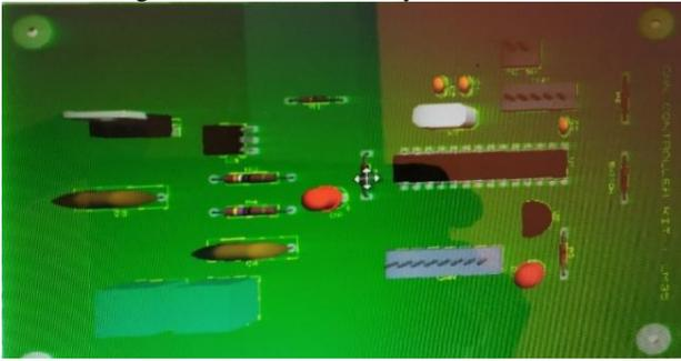
Figure 5: Board for temperature sensor with CAN and AVR interfacing
