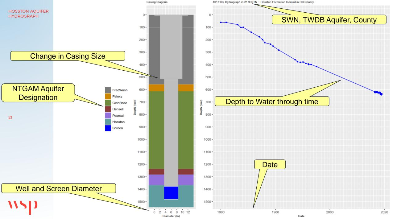
The Aquiter layers shown in the casing diagram were developed using the NTWGAM. In certain cases, assumptions used to develop the NTWGAM can cause well casing and screen intervals to not align well with modeled aquifer layers.
