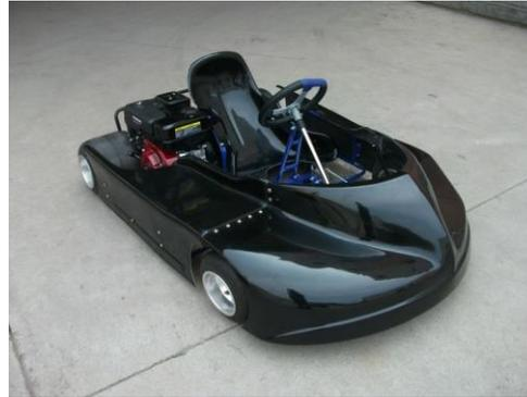
**Engine:** Must be a 196cc "Box Stock Clone" this must be as delivered from a parts supplier, no modifications are allowed. Billet flywheels are allowed. Recommended engine supplier and part number is [www.arcracing.com](http://www.arcracing.com) with their part number of DJ-1000 or DJ-1005.
