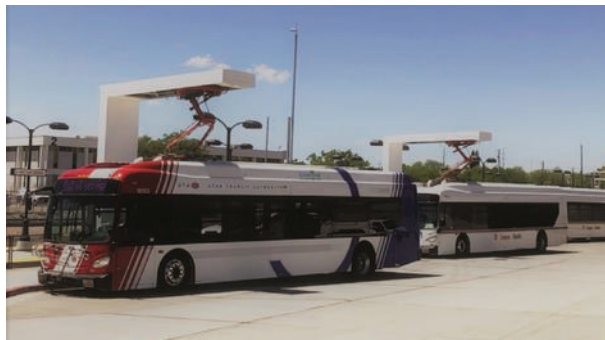
UTA electric buses charging at Salt Lake Central Station is one implementation of many planned electrification projects, several of which are being pursued in collaboration with Salt Lake City and the University of Utah.
