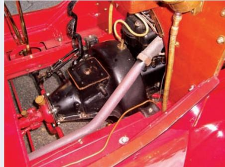
The reverse lever is positioned straight up in the top picture. Above, the roller follower is now in the lower cam step, indicating the clutch is released for 'neutral'. The clevis on the slow speed rod is provided for adjustment of the 'free neutral'.
