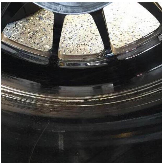
**Example of Scoring Damage on Caliper and Wheel**
