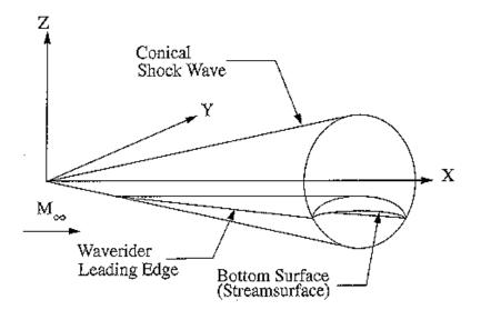
Figure 2-2. Conically Derived Waverider.
