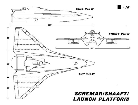
Figure 1-4. Schematic of Mated S<sup>3</sup> Platform (with SCREMAR).
