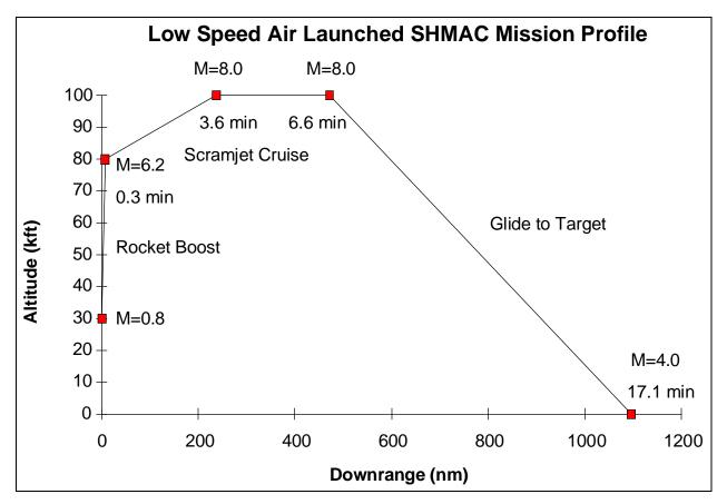
Figure 3-5. Low Speed Air Launched SHMAC Mission Profile.
