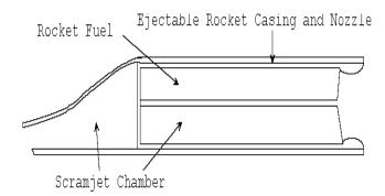
Figure 3-3. Rocket/Dump Combustor Scramjet.
