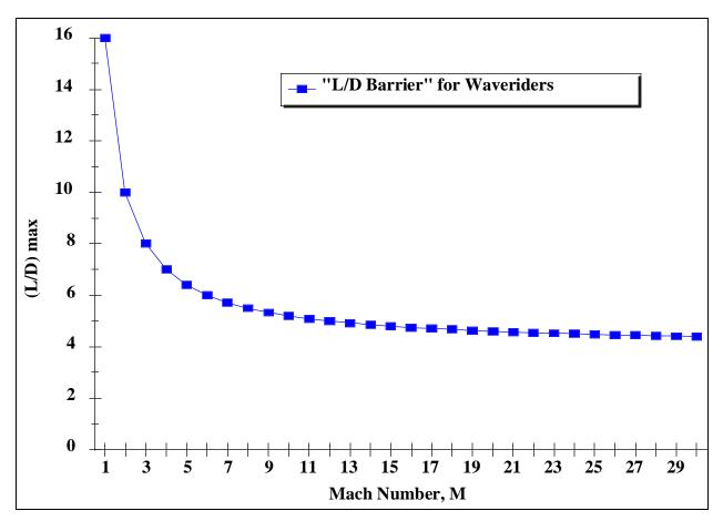
Figure 2-4. L/D Barrier for Waveriders.
