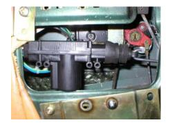
A pistol-style, 5-wire actuator getting installed in the front door of a RR Classic. You may have to try a few different positions (using the original mounting
