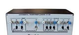
Model H-ET-100 Transformer utilizes a double-wound. multi-tapped, single-phase transformer. Binding taps are protected against overload by toggle-handled circuit breakers.
