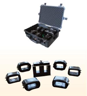
Model 1290B-6C Dissectible Transformer is a versatile device for teaching transform principles. The unit consists of a dissectible core and a complement of separate coils. An assortment of core gap spacers are provided for operation as a choke or reactor.
