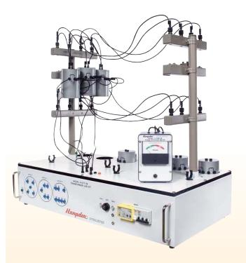
Model **H-DTT-26** Transformer Lab Kit allows students to make simulated connections to power transformers located on utility poles using miniature hardware. The upper three wires will represent the high voltage line (an optional 4th wire, representing a common neutral is also supplied), the lower three wires (4 wires for some configurations) will represent the service voltages from the transformer to the customer's secondary connections. Low voltage outputs provide a safe environment.
