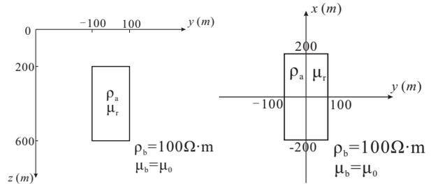
**Figure 2.** Cross section (left panel) and plane view (right panel) of the tested model used by validation and synthetic studies.
