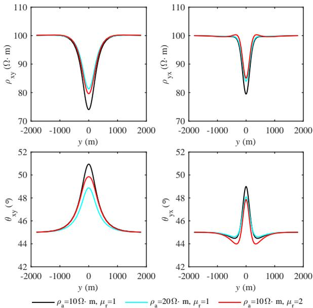
**Figure 4.** Magnetic effects on magnetotelluric forward responses of a conductive anomaly.
