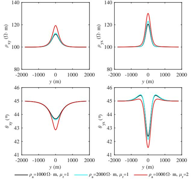
**Figure 5.** Magnetic effects on magnetotelluric forward responses of a resistive anomaly.
