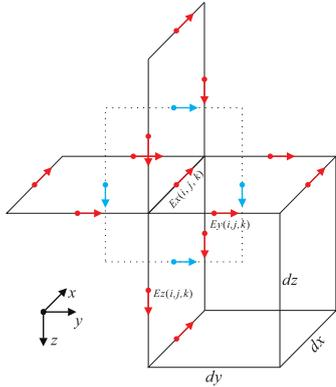
**Figure 1.** Demonstration for the coupling Maxwell's equations on staggered grid in finite difference method for 3-D magnetotelluric forward modeling. The electric fields are sampled along the cell edges and presented as red arrows. The magnetic fields are sampled across the center of the cell faces and presented as light blue arrows. The magnetic fields are across the discontinuities, thus requiring averages of the magnetic permeability of the corresponding adjacent cells.
