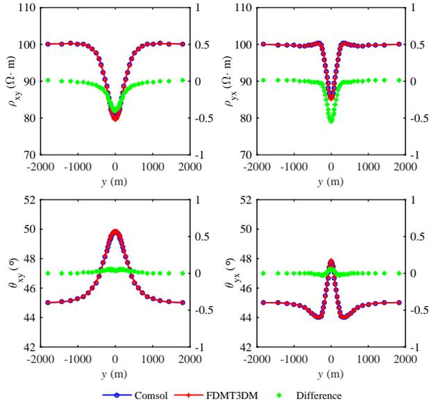
**Figure 3.** Comparing forward responses computed by our algorithm (FDMT3DM) with that by Comsol multiphysics. The differences between them are plotted in green dots and controlled by the right axis.
