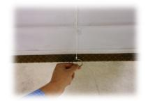
11. Check tension of spring and adjust by raising shade as far as it will go to the top, holding tube with one hand and turning adjuster wheel with the other (facing end of tube) counterclockwise to decrease and clockwise to increase tension. This should be adjusted before setting the stop.
