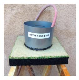
Test Procedure: An 18"x18"x3" MaxPour specimen was used to perform
