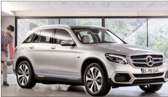
Mercedes-Benz is also showing preproduction models of its GLC F-CELL fuel cell plug-in hybrid. In addition to hydrogen, the all-electric variant of the popular SUV will also run on electricity. With 4.4 kg of hydrogen on board, the preproduction model produces enough energy for a range of up to 437 km (273 miles) in the NEDC, plus up to 49 km (27 miles) of all-electric range using its 13.8 kWh lithium-ion battery. Total output is 147 kW (197 hp) and top speed is electrically governed at 99 mph.
