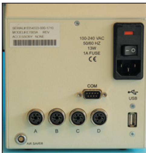
Accu-Touch rear panel connections.
