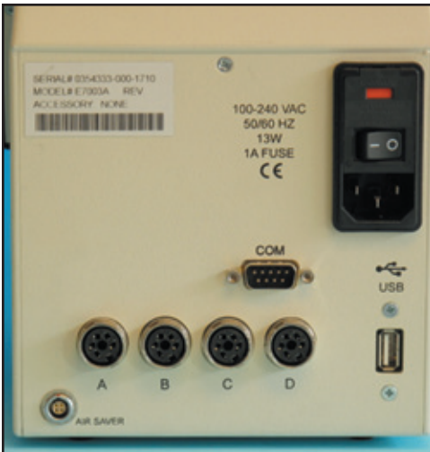
Accu-Touch rear panel connections.
