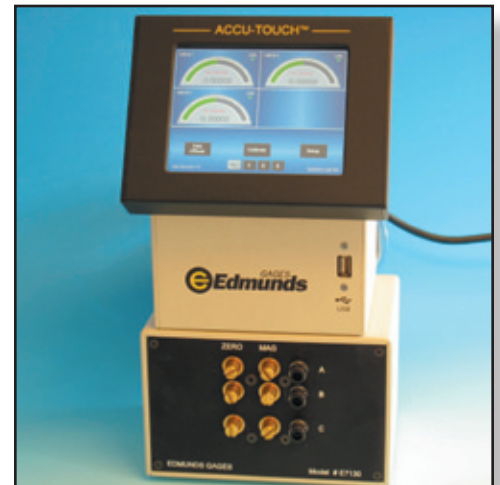
Accu-Touch 3-input docking air.
