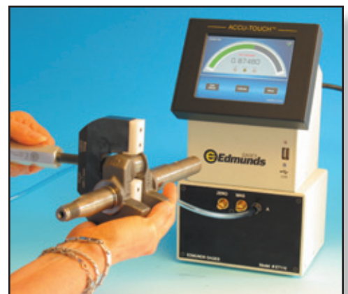
Real time display with inch, metric, absolute, or deviation.
