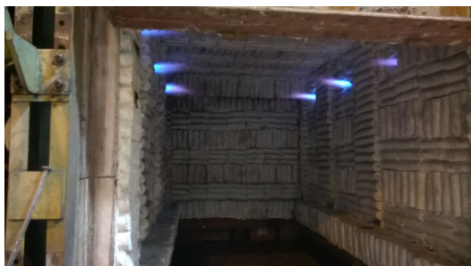
Complete rebuild replacing insulating firebrick using Crombie Industrial's custom manufactured ceramic fiber modules.
