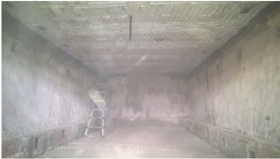
Crombie Industrial custom modules replacing an insulating firebrick ceiling, saving the customer thousands!
