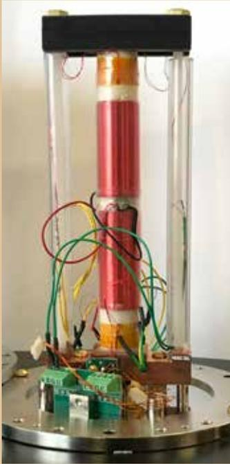
We use lock-in detection to process the signals, and thereby also become sensitive to electrical conductivity (if any), in addition to sensing magnetic susceptibility. We provide a suite of *samples* with the experiment; and in addition, we empower students to create their own samples, using an epoxy-encapsulation technique.
