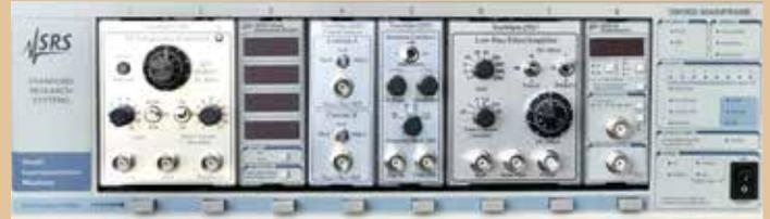
Stanford Research System's 'mainframe' for SIMs, populated with electronic modules from TeachSpin and SRS
