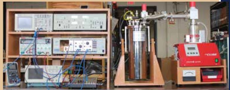
Support electronics on optional TeachSpin shelving (at left) accompanies the CMP dewar (center) and recommended pumping system (at right) to ~~fill~~ meters of table space.
