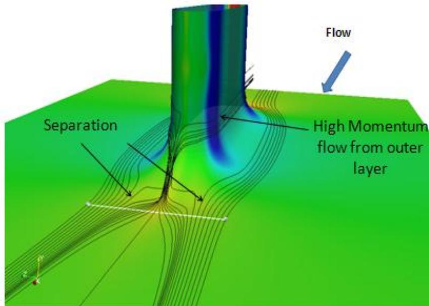
Streamlines around a scAUR™ fairing around a pier (5) with VorGAUR™ vortex generators (3) that produce no scouring vortices.
