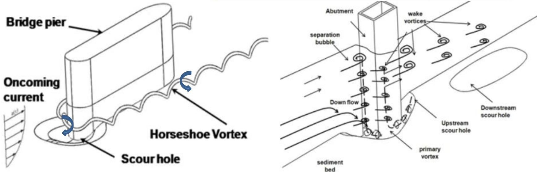
Bridge scour is produced by discrete vortices formed around unprotected piers (left above) and abutments (right).
