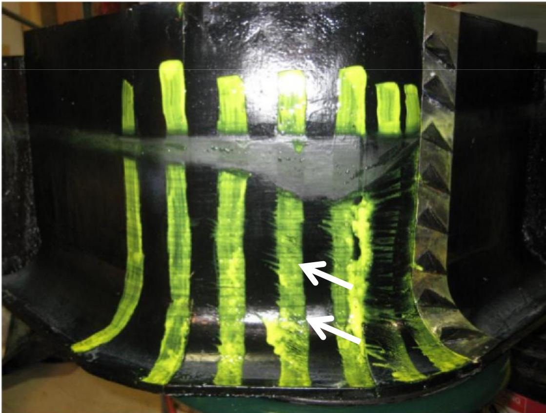
**Surface oilflow results for the case #20 modified wing-wall abutment model with VGs. The gray region is produced by a mixture of the oilflow material and waterborne substances at the free surface.**
