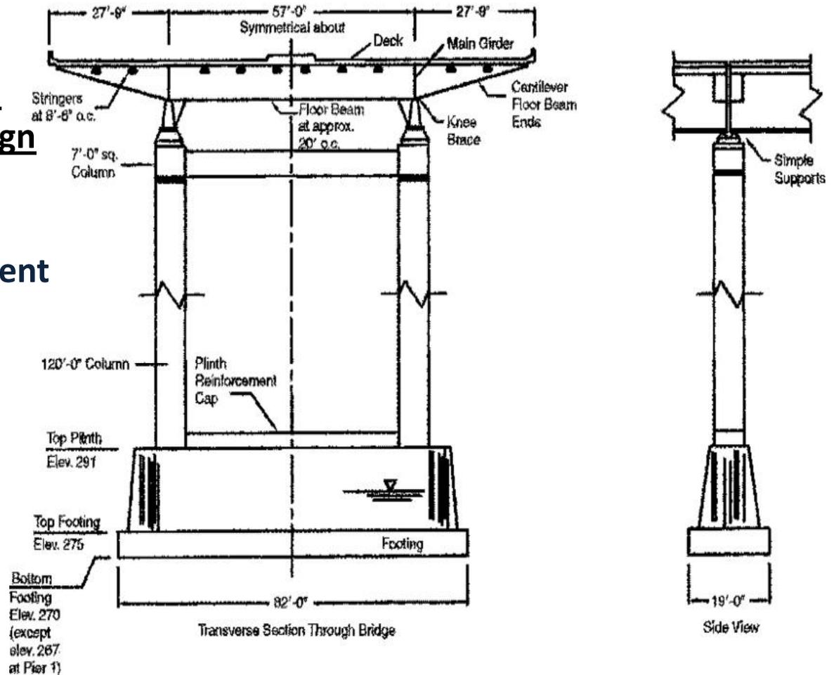
**Sections showing the Schoharie Creek Bridge pier supported on a spread footing . From NTSB, 1988.**
