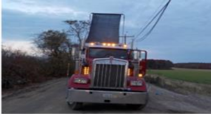
A truck driver was electrocuted when he tried to re-enter the truck's cab while the trailer's tarping mechanism was in contact with an energized overhead high-voltage power line.
