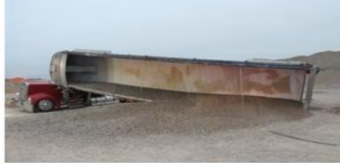
A truck driver died when his trailer tipped over onto the cab of the tractor. The driver was dumping part of the load of gravel from the trailer.
