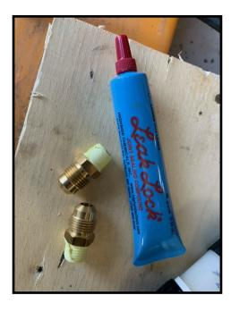
2. WRAP YELLOW GAS TAPE TIGHTLY AROUND THREADED 1/4" PART OF BRASS UNION THEN PUT JOINT COMPOUND AROUND THREADS. BE SURE NOT TO ALLOW ANY OF TAPE OR SEALANT TO BLOCK THE FLOW OF GAS
