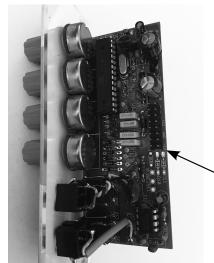
**NOTE:** Polarity is marked on the PCB board. Red stripe (-12v) facing downward.
