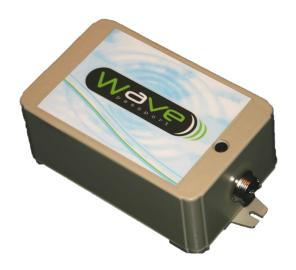
The WMR is an integrated device designed to securely and effectively read and send the information stored on RFID cards and keyfobs. Once captured, the unit communicates the ID information to the main computer or software and can be used to control any device associated with the reader such as an electric doorlock, turnstile, gate or any other electrically controlled system.
