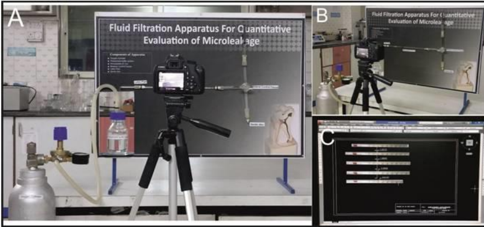
Fig 1: Showing the fluid filtration model. A-fluid filtration model with digital SLR camera .B. Lateral view. C. AutoCAD system (amount of bubble displacement).
