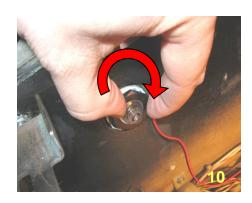
10. Apply the included plastic pal nuts to the button shafts, turning clockwise. They should be hand tight, but <u>do not use excessive force</u> as this can damage the LEDs. A very small amount of tightening with pliers can be used beyond hand tightening. But do not go much beyond hand tightening. The plastic nut fitment and notches in the cabinet will prevent the buttons from being loose or spinning.
