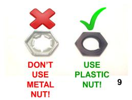
9. It is now time to fasten the LED ring and button to the cabinet using the included PLASTIC Pal nuts. IMPORTANT: DO NOT USE THE OLD METAL NUT TO SECURE YOUR LED BUTTON LIGHT. The metal Pal nuts can conduct electricity and short circuit the LEDs! Only use the included plastic Pal nuts to secure your LED ring and new button.
