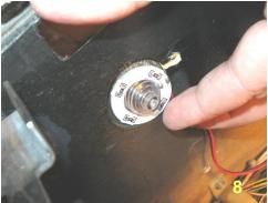
8. The LEDs are interchangeable, so either ring can be used on either side of the machine. Apply the LED ring over the shaft of the new button, making sure the 12 LEDs are facing in toward the button and the 4 resistors are facing outward toward the threads as shown.
