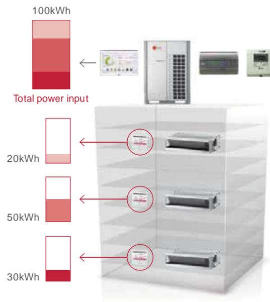
\* Outdoor unit's accumulated electric energy / using rate of individual indoor unit + indoor unit's accumulated electric energy is displayed in wired remote controller, only when central controller, digital integrating electricity meter and PDI are installed and PDI, outdoor unit and indoor unit are connected with power wire. Only total accumulated electric energy is displayed in standard wired remote controller. In premium wired remote controller, that are displayed into week / month / year.
