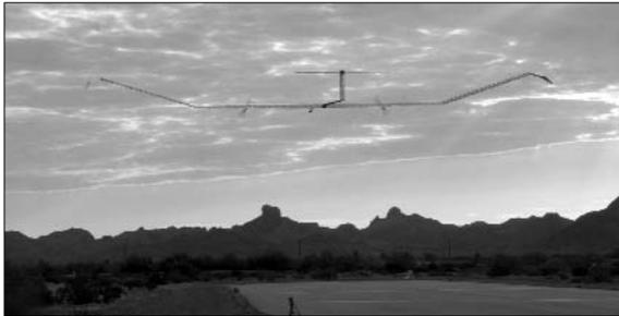
Some EVs can fly. A news story around mid-July was the Zephyr solar-powered electric airplane: On July 17 CNN reported that the unmanned plane, developed by UK defense company QinetiQ, took off from Yuma Proving Ground in Arizona on July 9 and was still in the air seven days later. The plane is equipped with lithium-sulfur batteries that allow it to fly at night.
