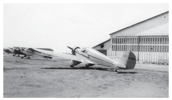
1935. The Aeronca Model K was to be an update of the C-3 design, with struts now bracing the wing and with a stilted mono-oleo landing gear, while the Model L was to be a new lowwing design that would use the same 40 hp. Aeronca E-113C engine.
