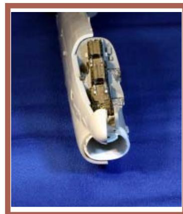
resin, they really help **PHOTO 1** with getting enough weight over the nose gear. I removed much of the floor and parts of side walls to get the metal seats to fit. I also had to extensively thin the bases of the metal seats. The seats were painted per web references. I wound the lower ejection pull handle from fine black and yellow wires.
