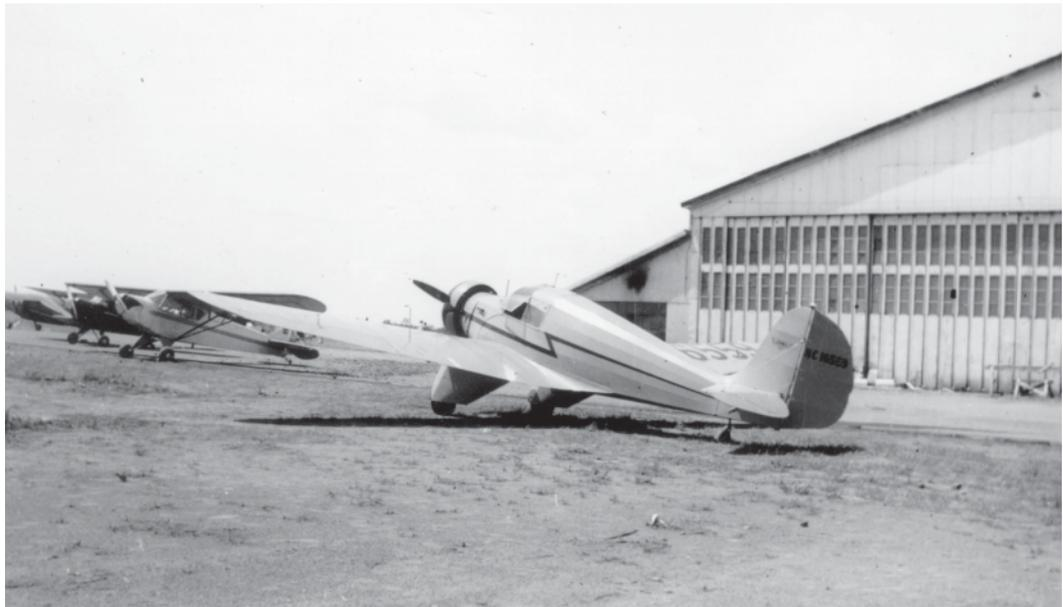
The subject of Tom's photo is manufacturer's serial number 2047. Registered as NC16559, it was one of only about 25 Aeronca LCs built, with the letter C indicating the substitution of a 90 hp. Warner Scarab engine. Unfortunately, there's no caption on the back of the original photo that might indicate when or
