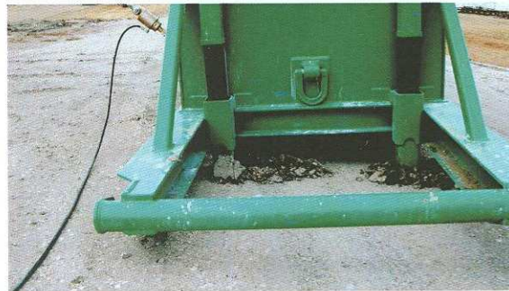
Dragging anchor along hard surface during side-pull test
