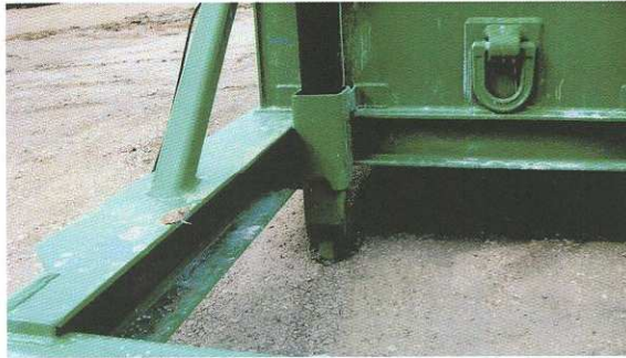
Hard-surface spikes penetrating hard surface
