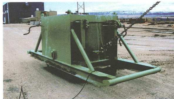
End-pull test on hard surface
