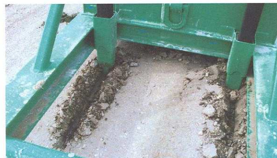
Dragging anchor along hard surface on end-pull test
