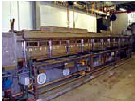
Steiner Tunnel Test
