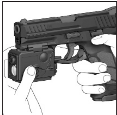
Figure 35 & 36 Installing accessory lights onto the rails
