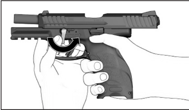
Figure 28 — Pivot the disassembly lever counter clockwise
