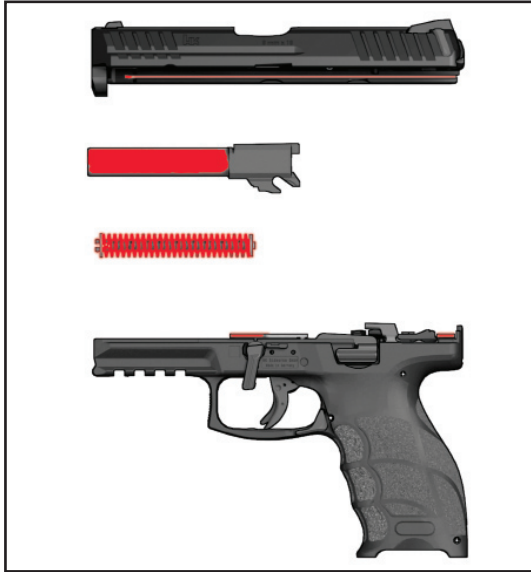
Figure 33 — Lubrications Points (in red)
