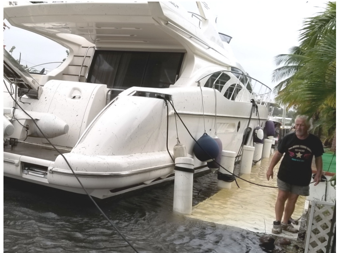
Dolphin Canal - Ken Stauch risks life and limb to add more lines to a neighbor's large yacht. Note how the first piling is leaning, as it had been pulled over by the yacht during the storm.
