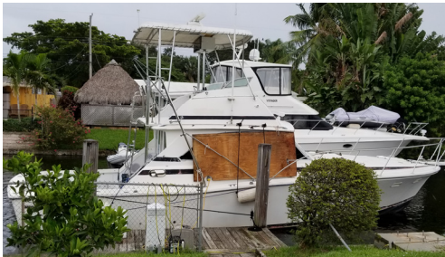
Ingenious design: Plywood hurricane shutters for boats
