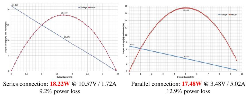
Circulating currents in the parallel case lead to increased Peltier effect and less power. 18
