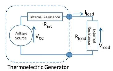
The Maximum Power Transfer Theorem states that when the load resistance equals the source resistance, exactly half of the electrical power generated by the TEG will be transferred to the external circuit. (Rest lost in Joule heat)
