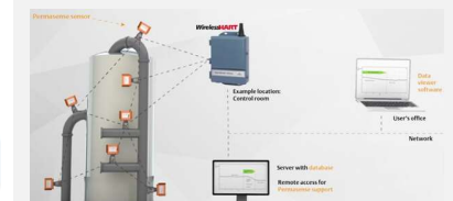
Rosemount Permasense Non-Intrusive Corrosion Monitoring
