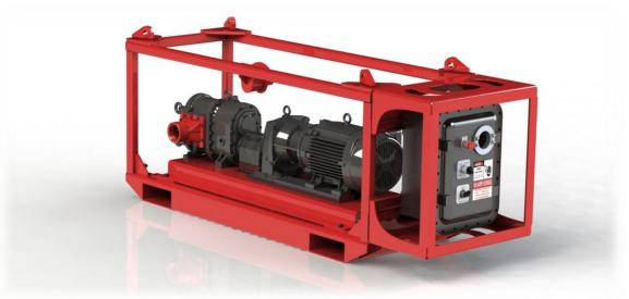
GTech USA supplies a vast variety of Rotary Lobe Positive Displacement Pumps on standard skid packages or customizable to suit your needs. These pumps are superior for pumping sludge, mud and thick fluids. The Maintenance in Place design allows for quick and convenient maintenance or replacement of all wear parts, without disconnecting from piping, drives or others components.
