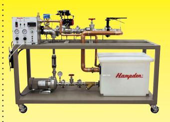
The Hampden **Model H-PVST-1** Pump and Valve System Trainer is a custom designed unit built to meet the plant specific training needs of the industrial facility. The trainer includes the basic facilities necessary to pump water (or other fluids) in a loop, together with the plant specific pump(s), valves and control configurations. Furthermore, all major components are flange fitted which allows easy removal from the unit. This will enable the trainee to learn the proper service procedures.
