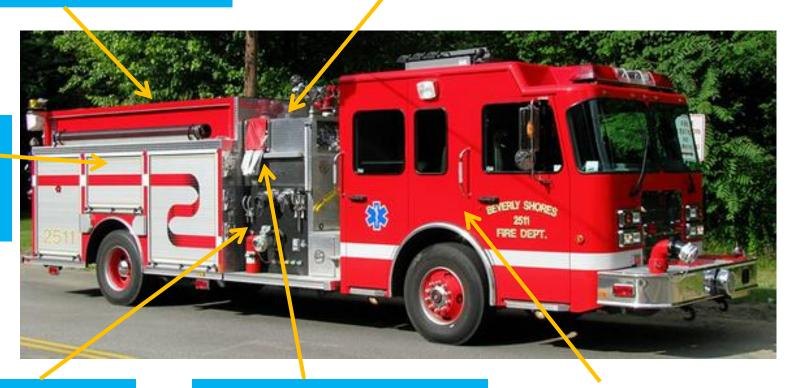
1750 gpm pump. Engine Water to Fire. 2 – 200' Cross Lay 1 ¾ "
