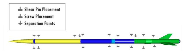
Each color indicates an independent section. The blue collar on the left shows where the payload will be stowed.
