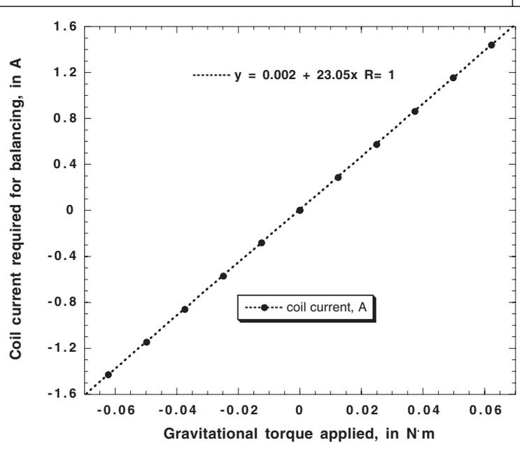
Fig 2: The current required to balance out a given gravitational torque
