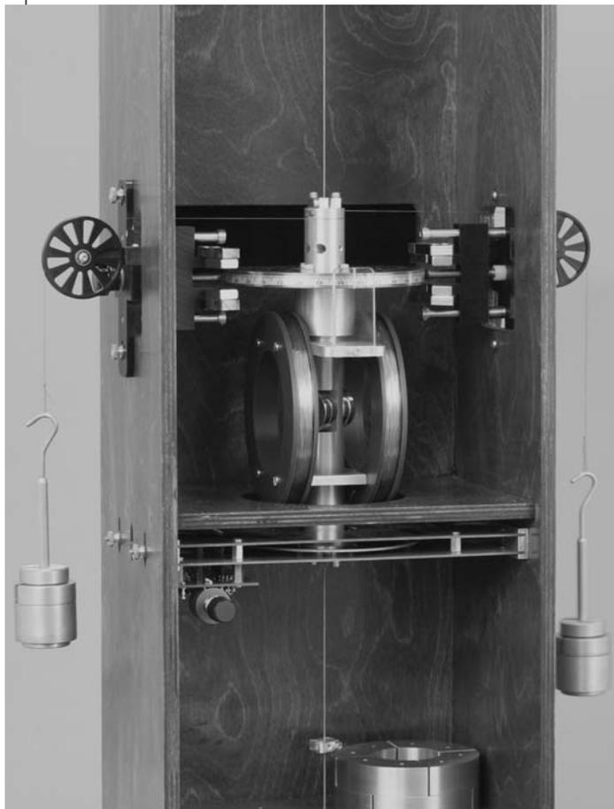
Fig 1: Center Section of the Torsional Oscillator
