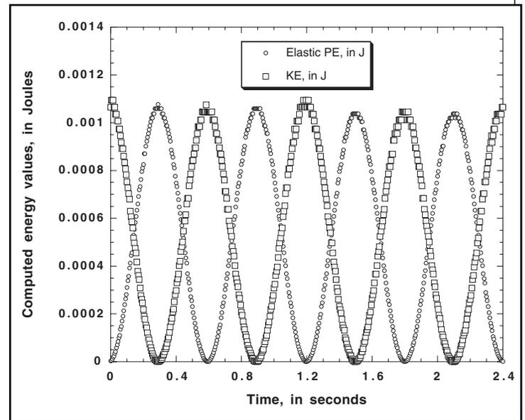
**Fig 6: Waveforms for kinetic and potential energy as functions of time, computed from the data of Fig. 5**
