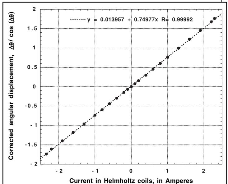
**Fig 4: The data of Fig. 3 re-plotted, showing the linear dependence of  $\Delta\theta/\cos(\Delta\theta)$  on coil current  $i$**
