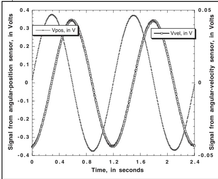
**Fig 5: Signals from the position sensor (left scale) and the velocity sensor (right scale) during simple harmonic motion**
