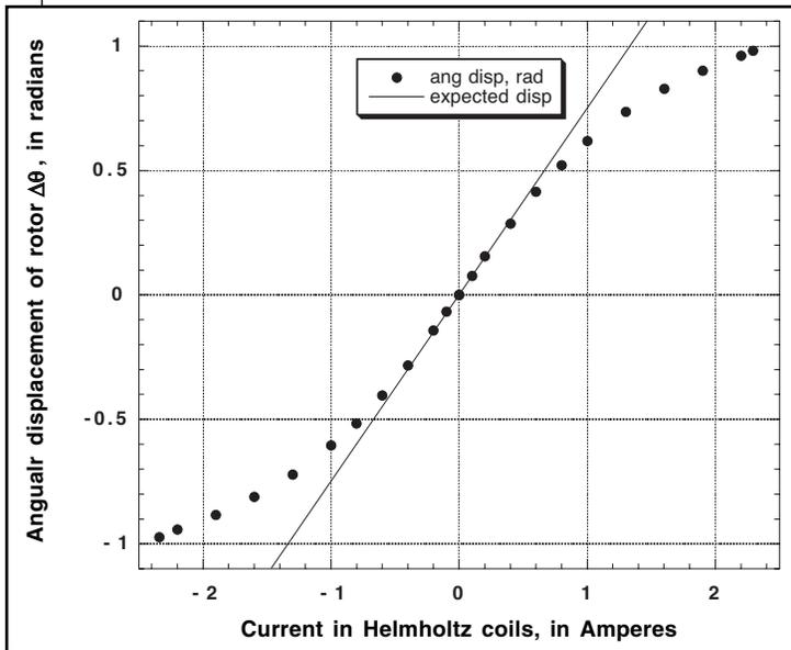
**Fig 3: Angular displacement  $\Delta\theta$  of the rotor from equilibrium, in response to magnetic torque arising from coil current  $i$**
