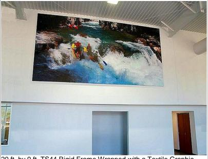
20 ft. by 9 ft. TS44 Rigid Frame Wrapped with a Textile Graphic fixed on the Rear of the Frame.
