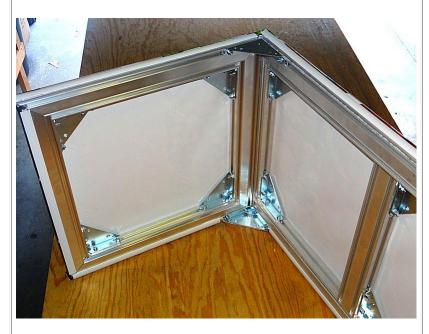
Here, you have a prototype fabricated for illustrating how to build a corner shape with the necessary hardware that we provide.
