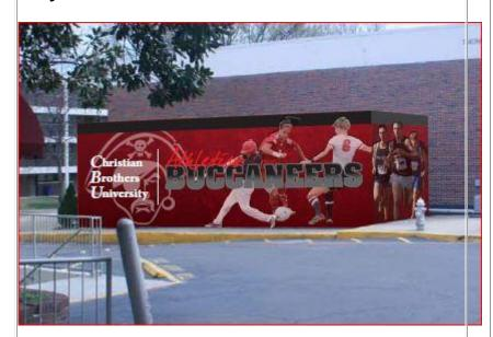
The TS44 extrusion is a great solution for outside structures temporarily hiding shop renovations for instance (Construction walls), or permanently hiding equipment, such as gas and water pipes, meters,... Here a U-shaped structure was built to hide pipes.
