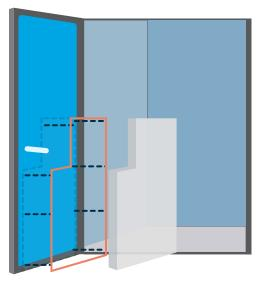
Position the Spacer Between the Space Guard and the door
