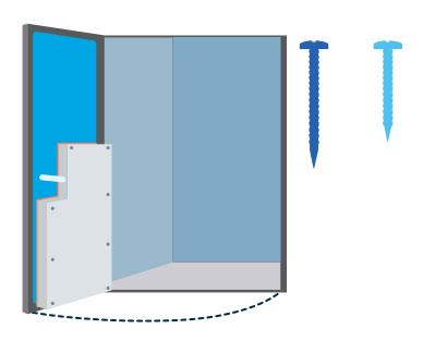
Close and open the door to make sure the space guard does not interfere with the door's operation.
