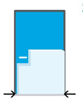
Position the space guard on the inside (hoistway) face of the door so that the bottom is flush with the bottom of the door.
