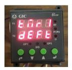
**Step 3:** Timer 1 Default Mode. Use the up and down arrows and select "00". This is "ON DELAY" Hit Enter
