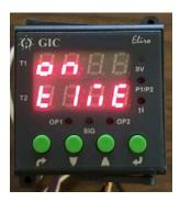
**Step 13:** Select Desired Forward Time Scale. Normally Hours and Minutes. Optional Minutes and Seconds. Hit Enter
