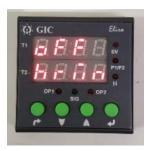
**Step 5:** Select the time for which the Reverse Cycle Runs. This is currently set to 30 minutes in this example. Use the up and down arrows to change this. Hit Enter
