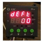
**Step 4:** Select Desired Reversing Time Scale. Normally Hours and Minutes. Optional Minutes and Seconds. Hit Enter
