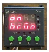
**Step 14:** Select the time for which the Forward Cycle Runs. This is currently set to 30 minutes in this example. Use the up and down arrows to change this. Hit Enter
