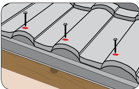
Fasten the bottom row panels through the top of the panel as shown, out of the main water channel of the panel. Top panel fastening is acceptable behind Boral Steel EZ-Vents and chimney/skylight details, as necessary.
