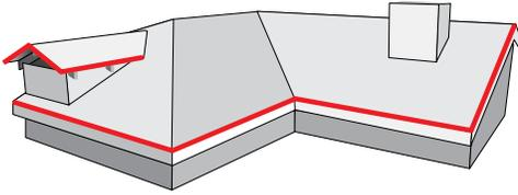
Install the BARREL-VAULT Tile Bird-Stop Riser across the fascia on top of a 1x4 Support Batten. The positioning is critical as this part will dictate panel layout across the roof, as the panels follow the scalloped profile of the Bird-Stop.
