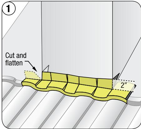
**1** At front of chimney, measure, cut and fold up panel up 2".
