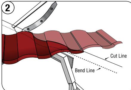
2 Mark the bend line 1 1/2" in from the cut line (1" bend down when installed Direct-to-Deck).
