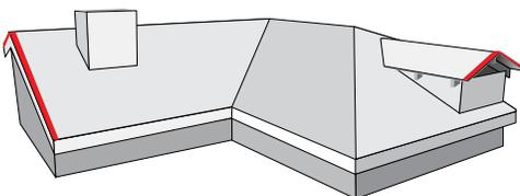
Measure, cut and install rake panel sections up each rake. Make sure to insert each section into the Rake Channel a min of .75". Refer to Panel Layout pages for correct panel lap and stagger layout.
