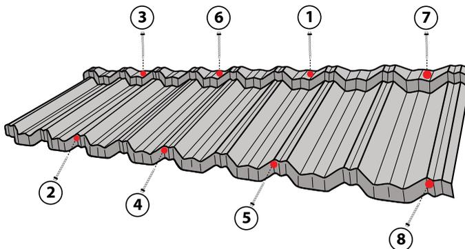
The fastening pattern for PACIFIC Tile uses four (4) fasteners across the front Nose Down-Turn and four (4) across the Back Top-Flange of each panel.
