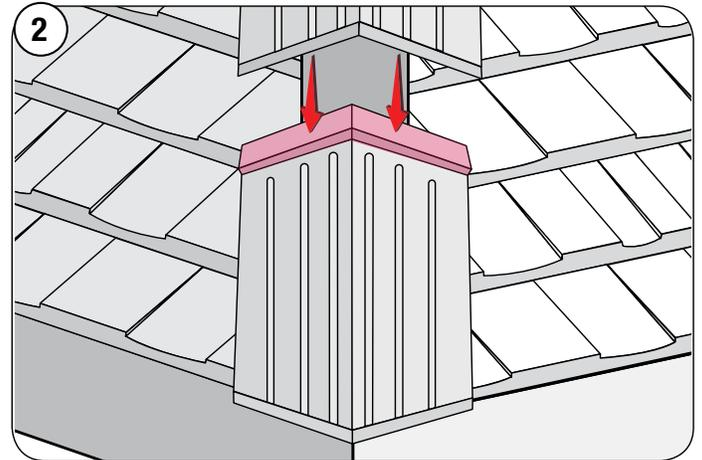
Position the Starter Cap at the fascia trimming the end to form a 3-D shape (Refer to hip starter cap detail Step 4 on page 21.)
