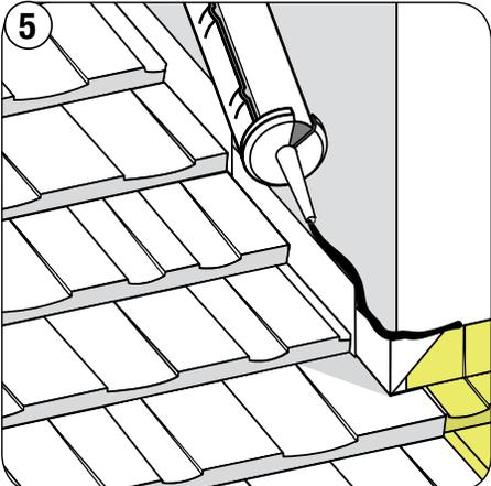
5 Seal around perimeter of folded panels prior to fastening to the protrusion.
