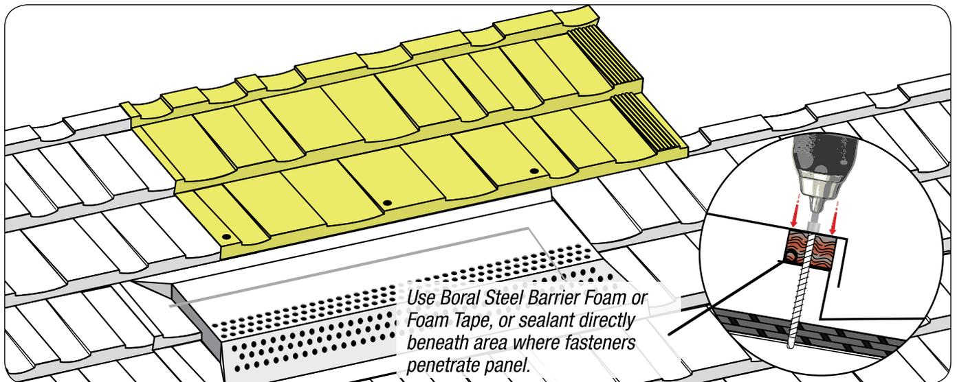
Top panel fastening is acceptable behind Boral Steel EZ-Vents, Chimney's & Skylights as long as they are positioned out of the main water channels on the high ribs of the panel. Fasteners should be covered with material from a Boral Steel Touch-Up Kit.
