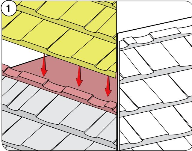
Optional accessory steel batten made from minimum 24 ga steel may be used to install caps on hips and ridges without the need to bend-up the panels. Steel battens require 2-pcs per each 10-ft length of hip or ridge. Steel accessory battens require the use of EmSeal foam tape or Barrier foam rolls under the batten.
