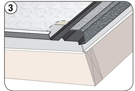
3 Install Gutter Riser across the fascia, underneath Underlayment and butt up against the Rake Channel and Valley pans.
