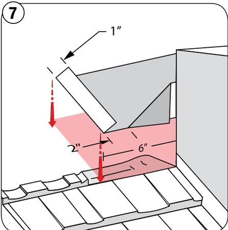
7 Install chimney saddle metal at back of chimney as shown. Extend saddle metal a minimum of 4" past each side of protrusion. Wakaflex® may be used as an option to form a chimney saddle around roof protrusions.
