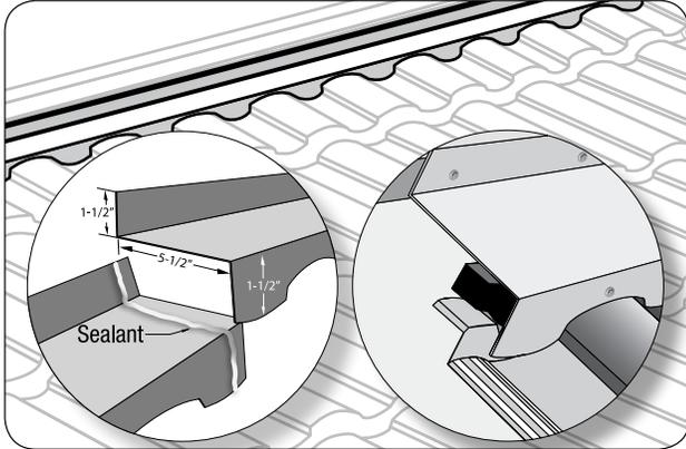
Apply a bead of Sealant between two overlapping Top Row pieces.
