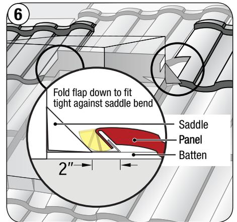
Install a section of Foam (debris block) across the chimney saddle as shown (align with BARREL-VAULT Tile profile).
