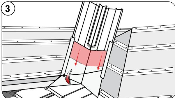
3 Install Valley metal over and onto the stone coated Flat Sheet. Apply a bead of sealant across the top of the Flat Sheet and embed the Valley into the sealant.
