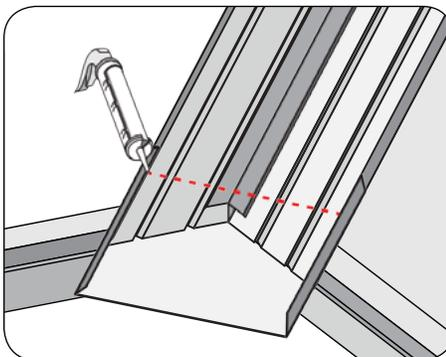
Apply a bead of sealant atop the Flat Sheet and seat the Valley Metal as shown.
