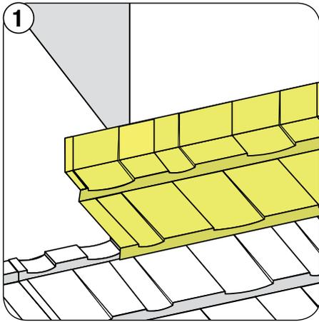
1 Measure, cut, and fold up panel 2" min. from the back of the panel to the front of protrusion.
