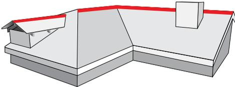
Measure, cut and install panels across ridge. Fasten as field panels. Overlapping panels is acceptable at the "horizontal" center line.
