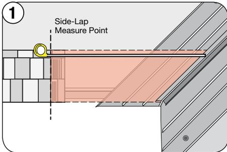
1 Measure from the Side-Lap reference point, mark & cut panels to fit into the Valley 2-Pc, matching the angle of the Valley.
