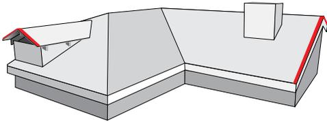
Boral Steel Trim Cap Rake Metal is installed along the rake edges as shown. This metal edging aids in positioning Boral Steel Trim Caps.
