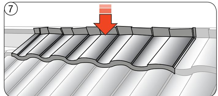
Force back of panel into position against ridge batten before fastening
