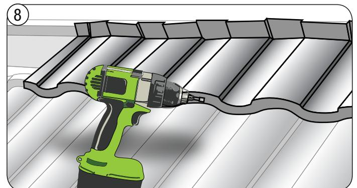
Fasten Ridge panel using four (4) fasteners across the nose (Refer to panel layout pages).
