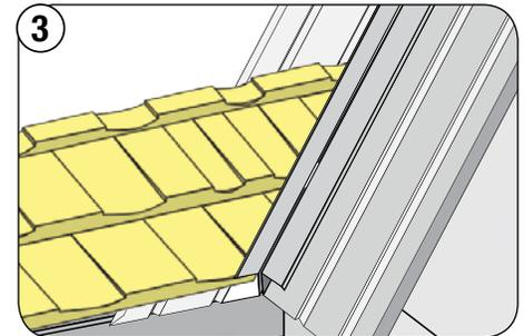
3 Valley panel cut & notched sections are fitted into the Valley 2-Pc as shown.
