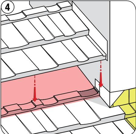
4 Install subsequent panels with a 2" bend up against the protrusion.
