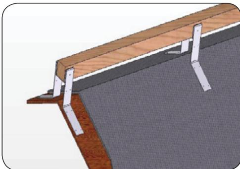
Install Ridge Riser Brackets no greater than 24 inches apart, place a 2"x 2" wood nailer board into Ridge Riser Brackets. Fasten wood nailer to Ridge Riser Brackets with a #8 min. 3/4 inch screw or roofing nail.
