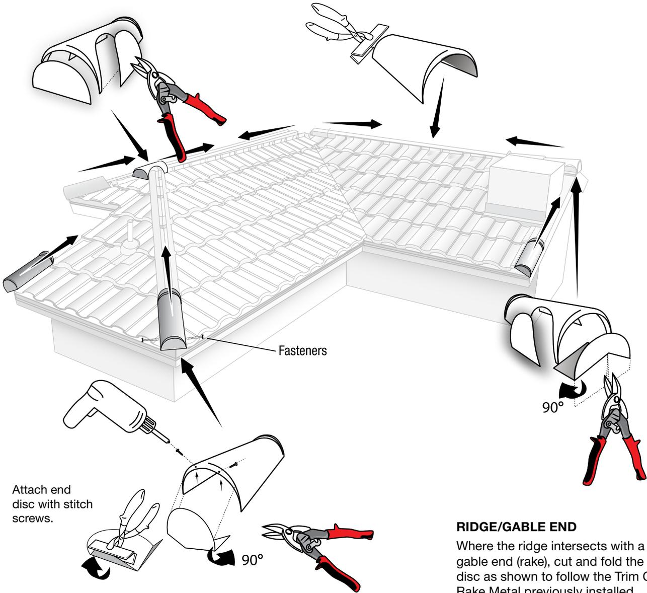
Attach end disc with stitch screws.
