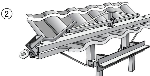
Always bend the ridge panels before cutting as they deform slightly in the bender. Deduct 1/2" from measurements. Mark both bend, and cut lines for each panel prior to cutting or bending.
