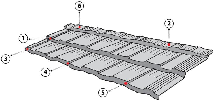
The fastening pattern for COTTAGE Shingle uses three (3) fasteners across the front Nose Down-Turn, two (2) fasteners across the Back Top-Flange and one (1) fastener on the Middle Nose Down-Turn of each panel.
