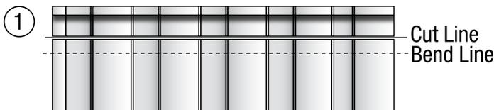
Ridge cut line is 2" above and parallel to bend line to allow for bend up on ridge battens.
