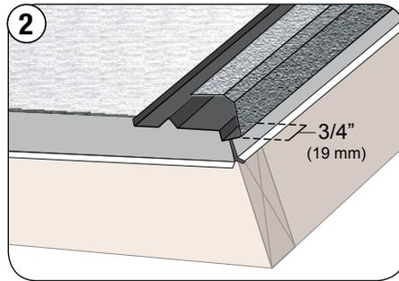
2 Install the Rake Channel up the rake extending it past the fascia Drip Edge by 3/4" (19 mm). Make sure the 'Locator-Lip' is snug against the rake Drip Edge and fasten with washer & grommet screws or apply sealant to screws.
