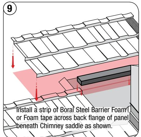
9 Install a strip of Boral Steel Barrier Foam or Foam tape across back flange of panel beneath Chimney saddle as shown. For added protection install a foam weather block under the panel overlapping the saddle.
