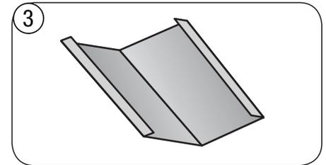
Hem both sides of the folded Flat Sheet as shown to fit around outside edges of valley.
