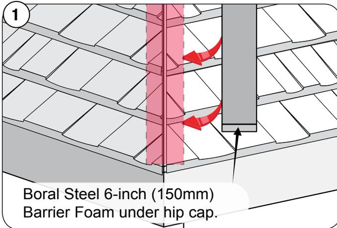
After cutting and installing panels to the Hip center-line, and creating a Hip Starter piece, apply Barrier Foam Roll (6" x 1" x 240") or butyl tape down center of hip, making sure the tape is seated on the panel surface at each panel course step.
