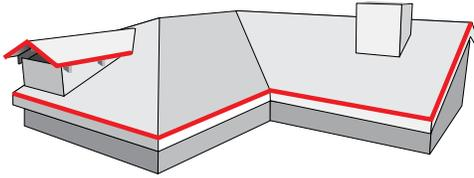
Boral Steel Direct-to-Deck panels are installed on new or existing roofs pitched a minimum of 3:12 (12 degrees). Underlayment is to be installed as per local code and manufacturer's instructions.
