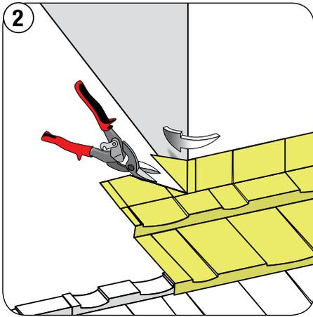
2 Cut a 45 degree angle as shown and fold tabs around protrusion.
