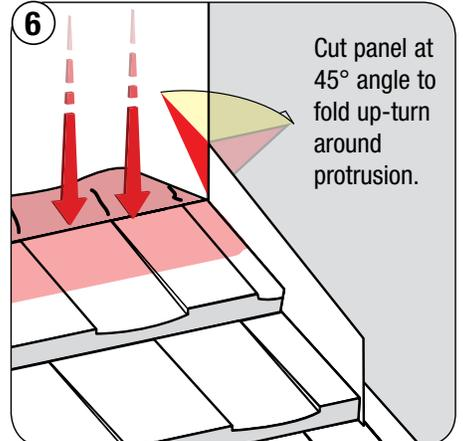
6 Flatten the back flange of the panel intersecting the top of the protrusion. Cut panel at 45° angle to fold up-turn around protrusion.
