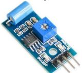
Fig.6 Vibration Sensor
