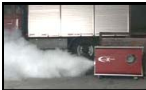
Figure 5 – Cold Smoke Test
