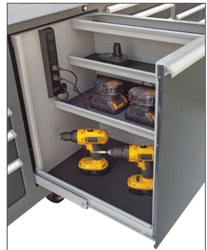
*The Power-Loc™ Drawer, for storage and charging of battery-powered tools.*
