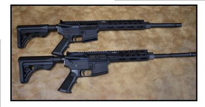
The Sagwu 5.56 or .300 blackout rifle is a standard AR Platform. The 16''  $1/2 \times 28$  (5/8 x 24 for .300 blackout) threaded
