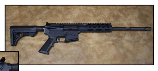
The Ta-li rifle is based on an AR platform. It accepts standard Glock style magazines with a straight blow-back action. The Ta-li rifle has a 16''  $1/2 \times 24$  threaded barrel. Standard features on a Ta-li rifle include: standard 4-position stock, free floated forearm, 17 round magazine, and 3-position ambi-safety marked with
