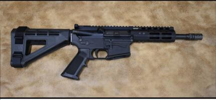
The Ta-li pistol is based on an AR platform. It accepts standard Glock style magazines with a straight blow-back
