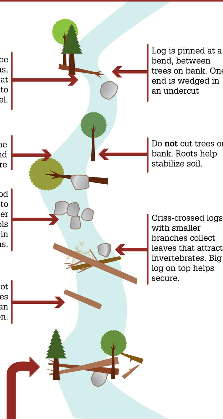
**Make a larger "strainer" every ~300 feet** to catch any loose logs from upstream.
