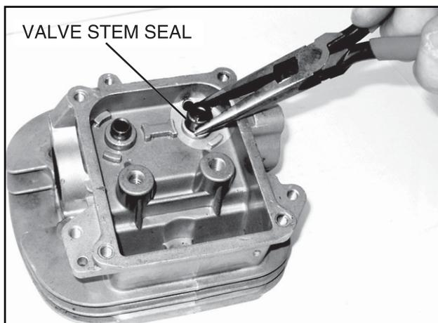
**Figure 5-6. Removing Valve Stem Seals**
