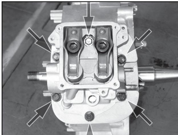
**Figure 5-4. Remove Cylinder Head**
