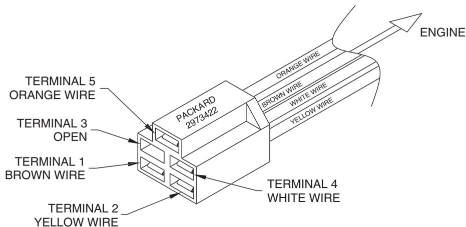
Figure 6-7. Optional Wire Harness Terminal Identification
