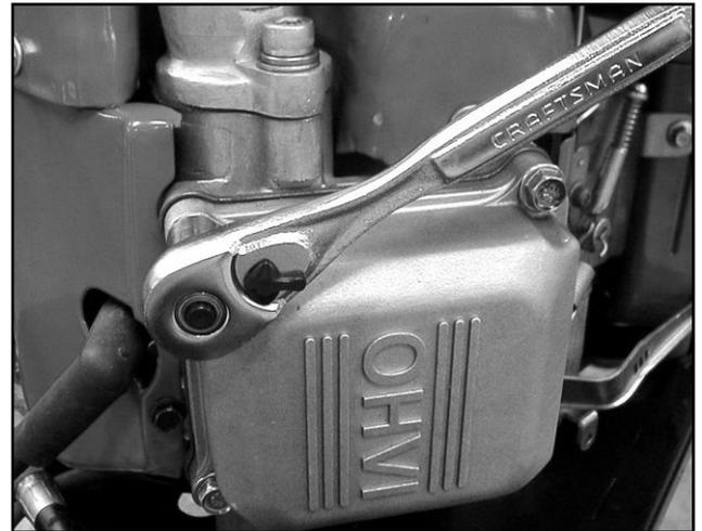
**Figure 5-18. Install Valve Covers**
