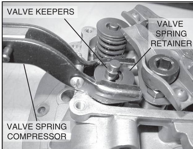
**Figure 5-5. Removing Retainers**
