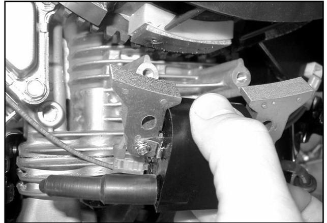
**Figure 2-1. Removing Armature**
