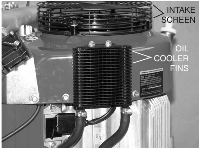
Figure 1-4. Clean Intake Screen & Oil Cooler Fins
