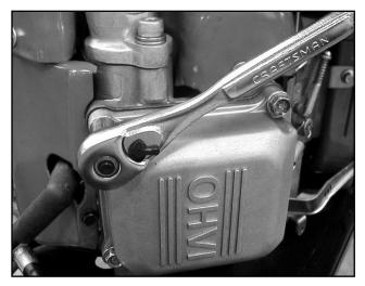
Figure 5-18. Install Valve Covers
